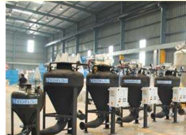
PNEUMATIC CONVEYING SYSTEM
